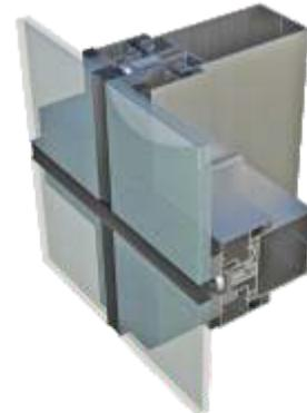
The profiles are sealed each other by a gasket system which controls the water entrance and conduction to the exterior weeping system, providing R650 level for water penetration in curtain walls, according to ASTM E331 and EN 12208 and C3 level for structural performance according to ASTM E330 and EN 12207.
